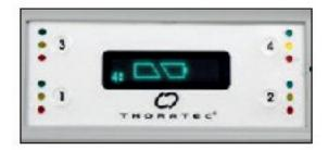
When calibration is complete, the yellow light turns off and the green light comes on, indicating that the battery is fully charged and ready for use.
