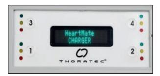
Each battery pocket on the charger has an associated set of lights: green, yellow and red. The light illuminated next to the battery pocket indicates the charge status of the battery:
