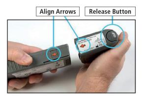
Procedure for moving from mains power to batteries:
