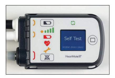
To initiate the self test press and hold the **Battery** button for five seconds. Then release the Battery button.
