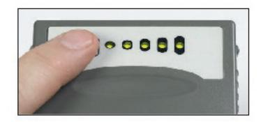
The number of bars illuminated on the battery gauge indicates the level of charge:
