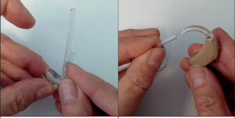
7. Take the old piece of tubing you saved and line it up with the newly threaded tube. Cut the end to the same length.
